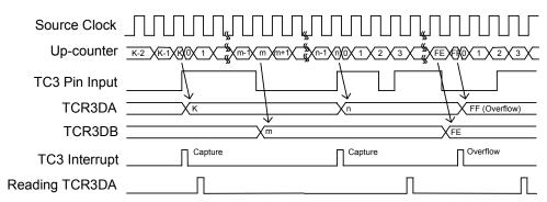
Fig. 24. Timing Chart of Capture Mode
